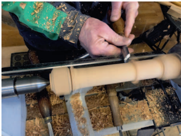
above, one of Toms 'bendy' pieces left, planing the surface with the spindle gouge
